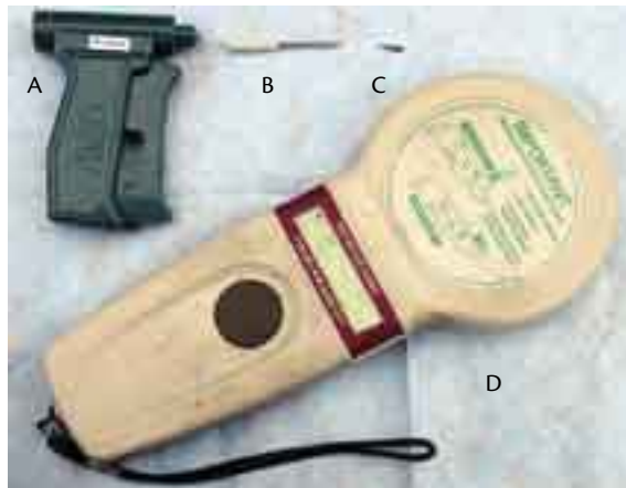
Figure 7.8 A passive integrated transponder (PIT) injector (A) with needle (B) and PIT tag (C), and a hand-held reading device (D).
