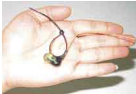
Figure 7.2 A radio-transmitter fitted to a plastic collar. This transmitter and collar set is suitable for attachment to a rat-sized rodent such as Rattus argentiventer or Bandicota bengalensis .
